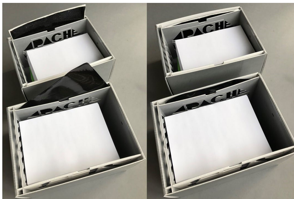
Figure 6. P2C boxes filled with paper and equipped with a PVA/GO board (top) and with a PVA/GO plate (bottom).
